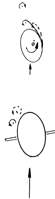
Fig. 16 Conceptual moving-wall effect on forebody flow separation and vortex development.
